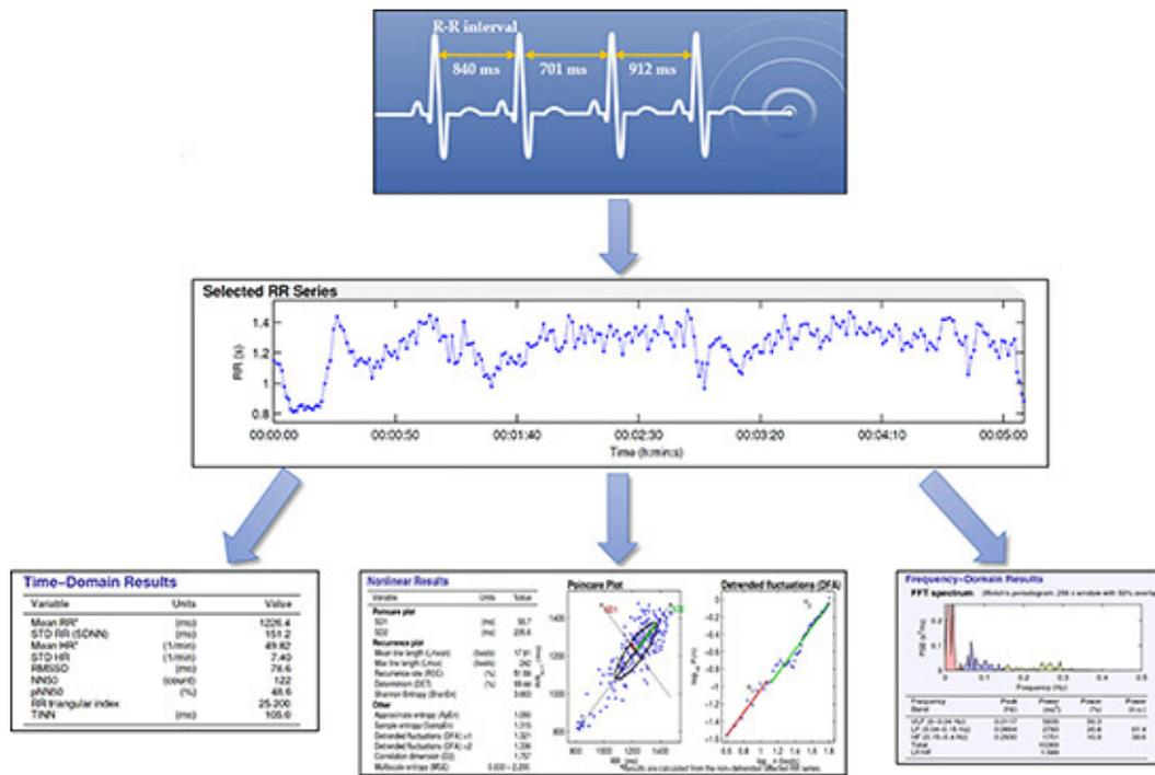
**Figure 5: Heart rate variability analysis. After proper identification of RR intervals from electrocardiogram trace (top picture), the measured time of each RR interval is plotted over time (middle picture). From the selected RR series, three common methods of HRV analysis can be performed: time domain, nonlinear and frequency domain (three bottom pictures).**
